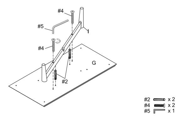
Step 7. Attach front leg frame (part H) to bottom panel (part G) by using large wood dowels (part #2), long bolts (part #4) and allen wrench (part #5).
