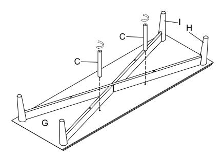
Step 9. Carefully turn the assembly over, and secure back leg frame (part I) and front leg frame (part H) to bottom panel (part G) by using bolts (part #3) and allen wrench (part #5).
