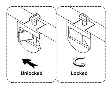
Reference the images above any time the instructions state "lock the hardware". Note: Be sure to check all hardware is locked when completed.
